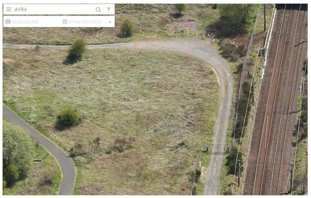
Parking/access area – Parking will be made just outside the access area. The parking and access area ground make up is of good condition, the access section at the track area consists of compacted gravel. The access area has discarded materials laying sporadically around the area. Site lighting will be required to highlight the hazards
