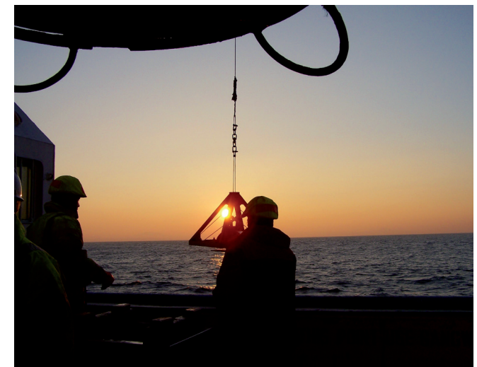
Figure 1: A day grab is used to collect sediment from the seabed for contaminant analysis. In this case the day grab was operated from the MRV Scotia.
