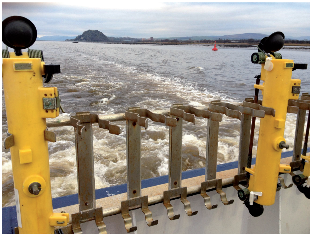
Figure 1: Water samplers used for taking samples in the Clyde estuary
